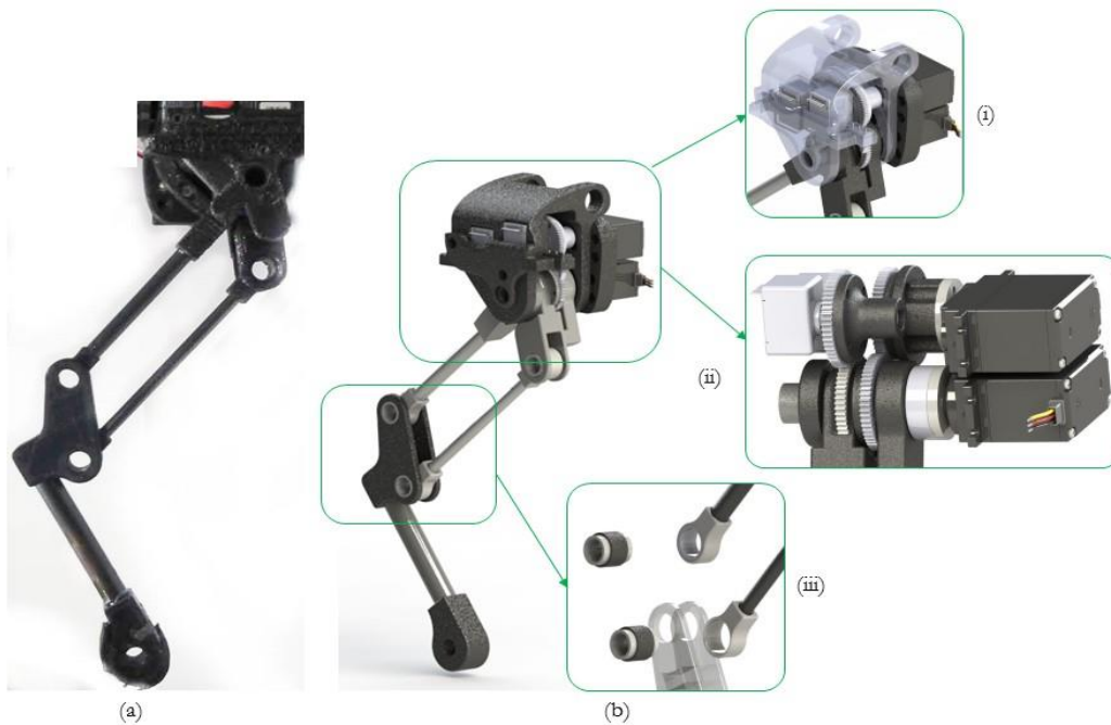
Figure 4. (a) shows the physical leg assembly, (b) shows the rendered counterpart of the leg assembly which has three parts: (i) sensor mounting and actuation hub, (ii) coupling and transmission of linkages with actuators and rotary encoders, and (iii) expexploded view of knee joint and CF journals.
