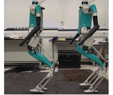
Fig. 5: Figures showing the disturbance rejection in torso pitch(left) and roll(center) upon the application of adversarial forces on Digit along the longitudinal and lateral axis respectively. The figure on the right shows the experimental setup where we performed preliminary transfer of the policy from simulation to hardware.
