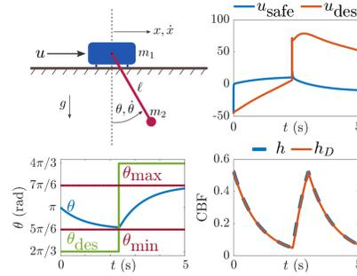
Fig. 4. Cart-pole system with energy-based CBF.
