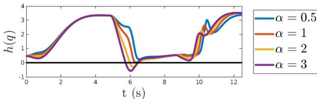
**Fig. 2.** Velocity-based kinematic barrier function on the 6 DOF manipulator. Safety depends on choice of  $\alpha$ . The times to complete these tasks are shown in the video [1] and listed in Fig. 3.
