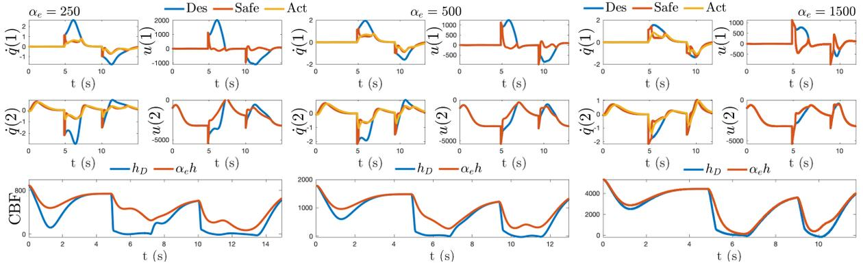
**Fig. 3.** Energy-based kinematic CBF on the 6 DOF manipulator. Safety is guaranteed regardless of the choice of  $\alpha_e$ , but performance improves as  $\alpha_e$  increases. The times taken to complete the second portion of the task, near the obstacle, are 10.07, 8.06, and 6.86 sec for  $\alpha_e = \{250, 500, 1500\}$ , compared to values of 7.60 to 7.94 for the purely kinematic case and 5.79 for CBF-free case. See video [1].
