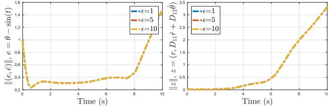
Fig. 2. Figures showing the PD tracking results as a function of time for the pendulum-slider system. All positions are in radians. See Fig. 1 for the pictorial representation of this system. Gravity is ignored for convenience.
