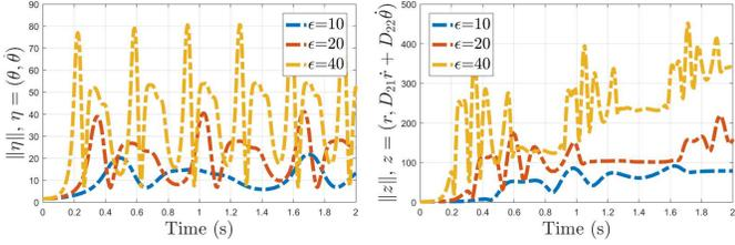
Fig. 3. Figures showing the tracking results for the cart-pole system. Position errors are measured in radians. See Fig. 1 for the pictorial representation of this system. Note that  $\eta = (\theta, \dot{\theta})$ .
