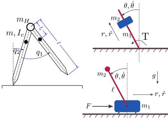
Fig. 1. Figure showing some examples of underactuated systems: the acrobot (left), the pendulum-slider (top right), and the cart-pole system (bottom right).
